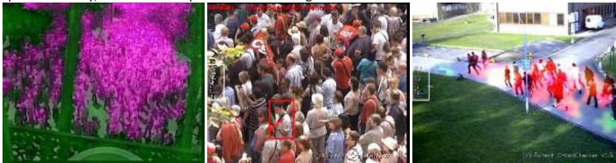
Figure 6 : (a) density map, (b) man crossing the crowd flow, (c) sudden crowd acceleration
