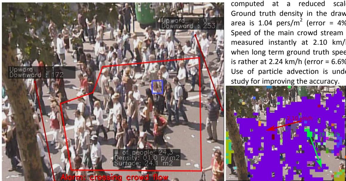
Figure 7 : (a) simultaneous density estimation, counting, and detection, (b) speed and direction
